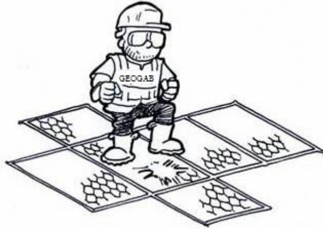
Unfolded gabion baskets panels
